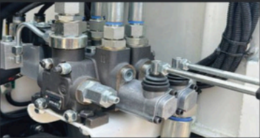
Manual operation for Emergency.
