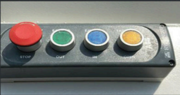
Ejector plate with IN/OUT functions and Emergency Stop.
