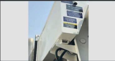
Hydraulic oil tank with filters.
