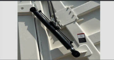
Tail gate lifting cylinders Heavy duty.
