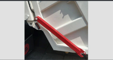
Maintenance lock for safety.
