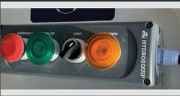
Bin lifter operation by buttons.
