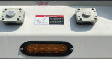
Tail gate lifting with 2 button safe operation
