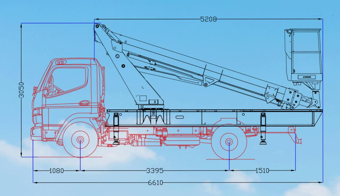
\*outreach and height max values and repeatability can change within ± 3% due to manufacturing variation and working condition
