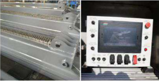
Lifting arm uses plate chain and arm status display system
