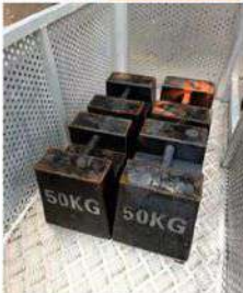
Strict overload test procedures, dynamic overload 125%, static overload 150% no problems occurred in the natural environment
