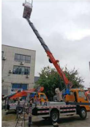
Strict overload test procedures, dynamic overload 125%, static overload 150%, no problems occurred in the natural environment
