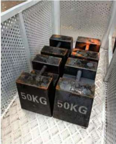
Strict overload test procedures, dynamic overload 125%, static overload 150%, no problems occurred in the natural environment
