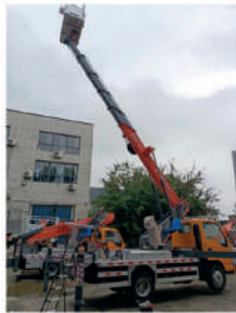
Strict overload test procedures, dynamic overload 125%, static overload 150% no problems occurred in the natural environment
