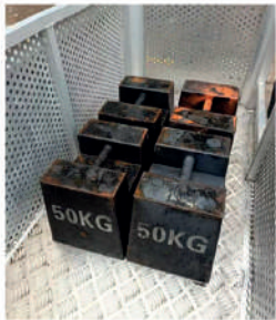
Strict overload test procedures, dynamic overload 125%, static overload 150% no problems occurred in the natural environment
