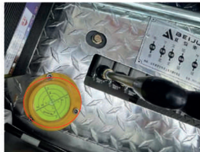
Level meter monitors balance status in real time
