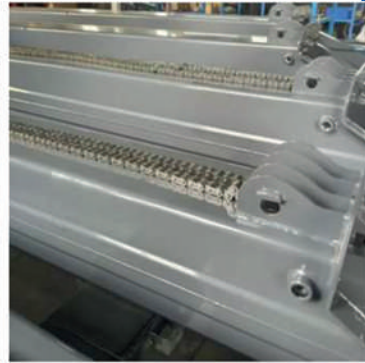
Lifting arm uses plate chain and arm status display system
