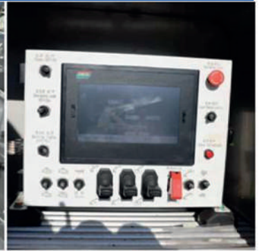
Lifting arm uses plate chain and arm status display system
