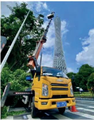
Strict overload test procedures, dynamic overload 125%, static overload 150% no problems occurred in the natural environment
